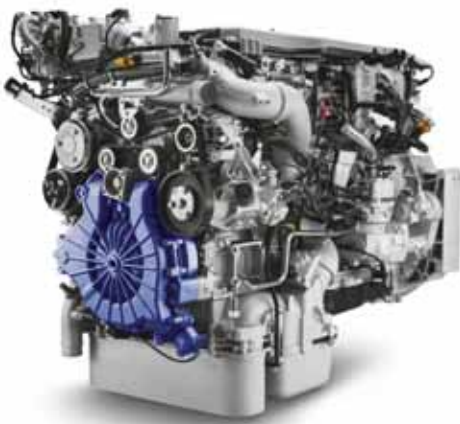
Aquatarder attached to engine front end
